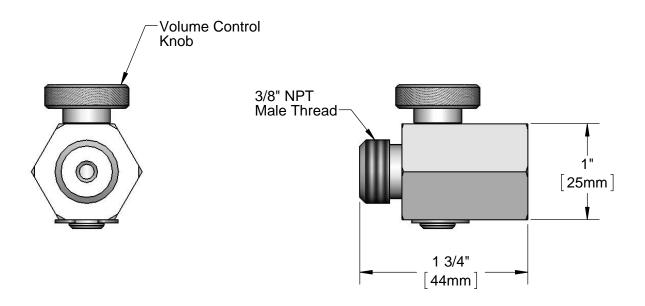
Flow Rate Adjustable From 0.1 gpm to 3.0 gpm, Based Upon 60 psi Water Pressure
