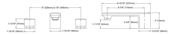
IMPORTANT NOTE: This valve/trim can only be installed in a built-up deck. It cannot be installed on pre-finished deck or on tub rim.
