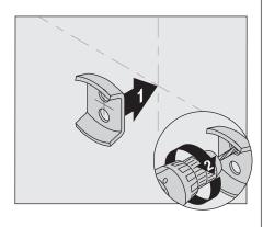
With mounting brackets in position, secure to wall using screws.
