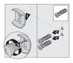
2b) **Stud Option:** Place mounting brackets into desired position. Using brackets as a guide, carefully drill 3/16" holes into wall.
