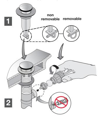
Step 7 Connect lift rod and adjust linkage
