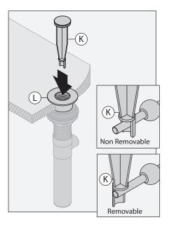
**Note:** Stopper can be installed removable or non-removable determined by eye hole position.
