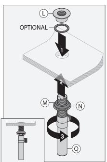
**Note:** Make sure drain cavity (on drain body) faces rear of sink.
