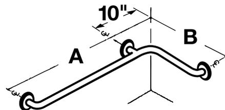
**General:** Furnish and install as shown on plans, Inside Corner-Style Safety Grab Bar model \_\_\_\_\_, as provided by E.L. Mustee & Sons, Inc. measuring \_\_\_x\_\_\_ with Twist-Lock concealed flange shall be 1-1/2" diameter, 18 gauge, type 304 stainless steel tubing. 14 gauge stainless steel mounting flange shall be Heliarc welded to the tube to form a single structural unit. Grab bar shall comply with applicable building codes. Meets ANSI A117.1
