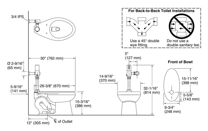
**Technical Information** All product dimensions are nominal. Toilet type: Floor-mount Waste Outlet: Floor Bowl shape: Elongated Flush type: Flushometer valve siphon Spud size: 1 1/2, Inlet, Top Trap passageway: 2-1/8" (54 mm) 10" x 7" (254 mm x 178 mm) Water surface size: Rim to water 6" (152 mm) surface: Rough-in: 12" (305 mm) Seat-mounting 5-1/2" (140 mm) holes:
