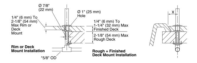
\* Indicates items to be supplied by installer. X= Distance from centerline of spout inlet to front of spout base plus 1/2" (13 mm).
