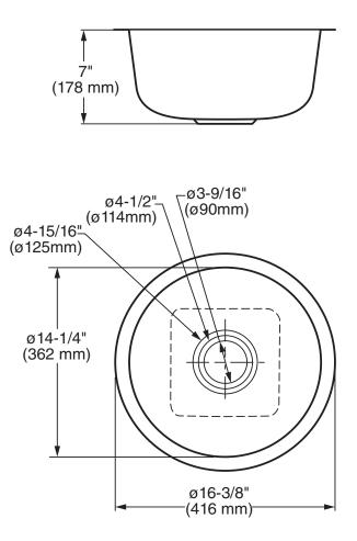
NOTES: \* DIMENSIONS SHOWN FOR LOCATION OF SUPPLIED AND "P" TRAP ARE SUGGESTED. FITTINGS NOT INCLUDED WITH FIXTURE AND MUST BE ORDERED SEPARATELY. SEALING COMPOUND SUPPLIED BY OTHERS.
