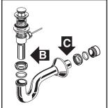
Connect water supplies lines and drain pipe connections. Turn water on and check for leaks.
