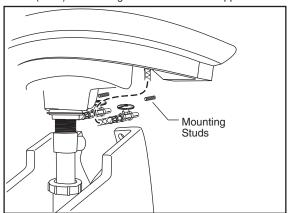
Through the access space between pedestal and lavatory use a 7/16" wrench to tighten the pedestal to wall.
