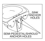
Drill (2) 9/32" dia. (7mm) holes 32" (813mm) up from finished floor, spaced at 4-3/4" (120.6mm) either side of centerline. Install (2) 3/8" x 4" (10mm x 102mm) lg studs using the double nut method, leaving 1-5/8" (41mm) of threaded end exposed. Mount the sink to studs temporarily, making sure the sink is level side to side.
