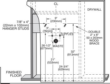
Position semi-pedestal under bottom lip of sink. While holding semi-pedestal in position reach through the access area between the lavatory and semi-pedestal and mark the location of anchor holes. Remove semi-pedestal and predrill 3/16" (4-5mm) dia. holes at locations marked. Install 1/4" x 3" lg studs leaving 1-1/4" exposed. Use same anchor screw installation as in 2a.
